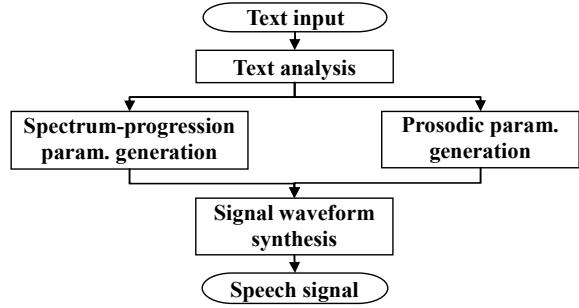
Fig. 5. System structure of our Mandarin synthesis system
