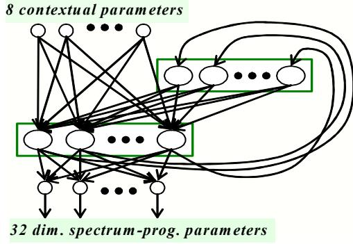
Fig. 4. ANN structure for spectrum progression modeling
