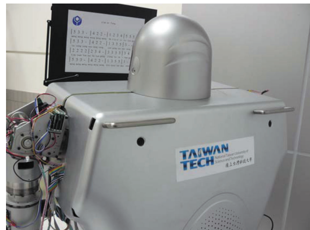
Fig. 15 The robot is reading the musical notations of the song and then singing it
